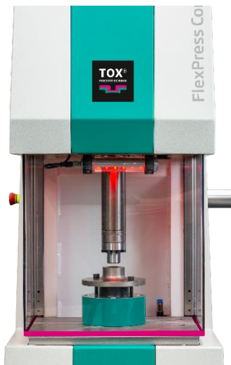
Image 2: The RGBW illumination of the work area lights up in red if the work process did not run correctly and the workpieces are not in order.
